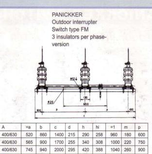
Fixing holes to customer's request Dimensions C and P adjustable to suit site conditions.
