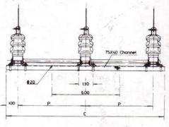
Fixing holes to customer's request Dimensions C and P adjustable to suit site conditions.
